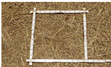
Example of adequate mulch coverage on 1sq.ft area. Photo credit: Maine DOT.
