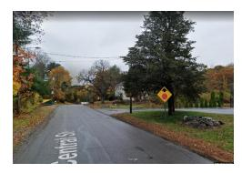
It does not appear a W3-1 sign exists on Glenn Ave. I recommend we install one about 500 feet in advance. On both side streets, we could also install additional W3-1 signs at 250 feet in advance, so drivers are reminded again of the stop condition ahead.
