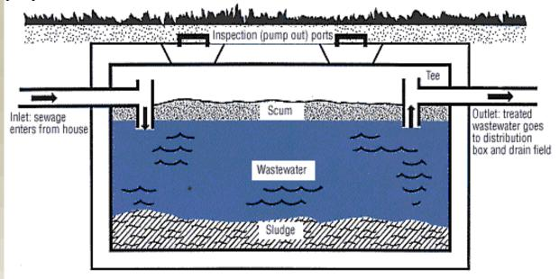
After partially treated wastewater leaves the tank, it flows into a distribution box, which separates this flow evenly into a network of drainfield trenches (shown on front cover). Drainage holes at the bottom of each line allow the wastewater to drain into gravel trenches for temporary storage. This effluent then slowly seeps into the subsurface soil where it is further treated and purified (secondary treatment). A properly functioning septic system does not pollute the groundwater.
